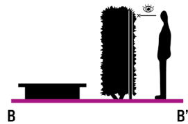
Figure 16: Metal fence with a height of approx. 1,60m, with a dense hawthorn hedge directly behind it, blocking the sightlines into the water extraction area.
